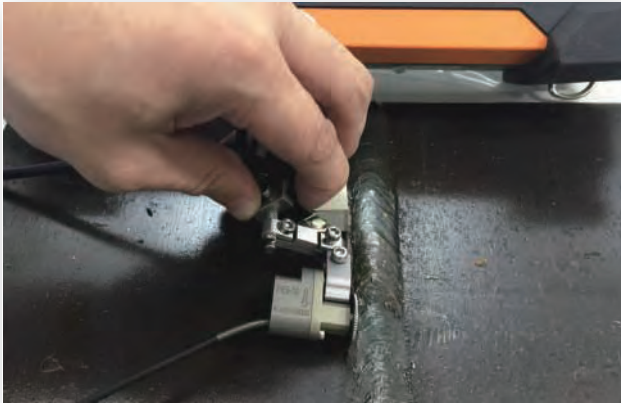
Butt Weld Inspection
