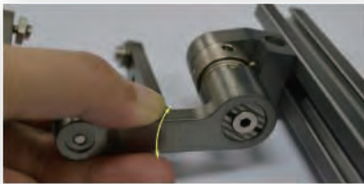
Turning Arm Adjustment
