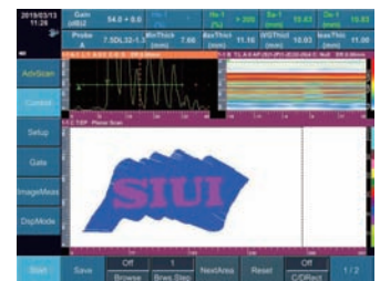
Corrosion C Scan
