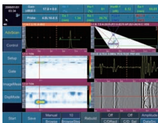
Simultaneous Inspection of PA & TOFD
