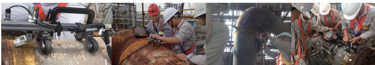
TOFD+Conventional UT to inspect blind zone area
